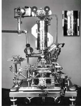
His #3 "Universal Microscope", completed in 1933, had 5,682 different parts and was capable of magnifying living objects (not dead on a slide) up to 60,000X their normal size.
